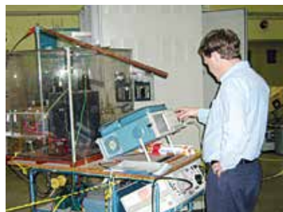
Imoulse Voltage Withstand Test
